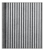
KSH-25 panels are linear ribbed lenses with a 90° included angle on 1/8" centers. A hammertone texture is applied to the lens surface to diffuse the light rays and eliminate harsh spikes of light.
