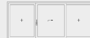
One lift/sliding sash and two fixed panes
