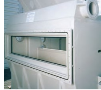
Industrial parts cleaner: SIMONA® PP homopolymer
